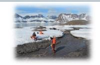
Phot. 37. Measurements of runoff from melting snow
